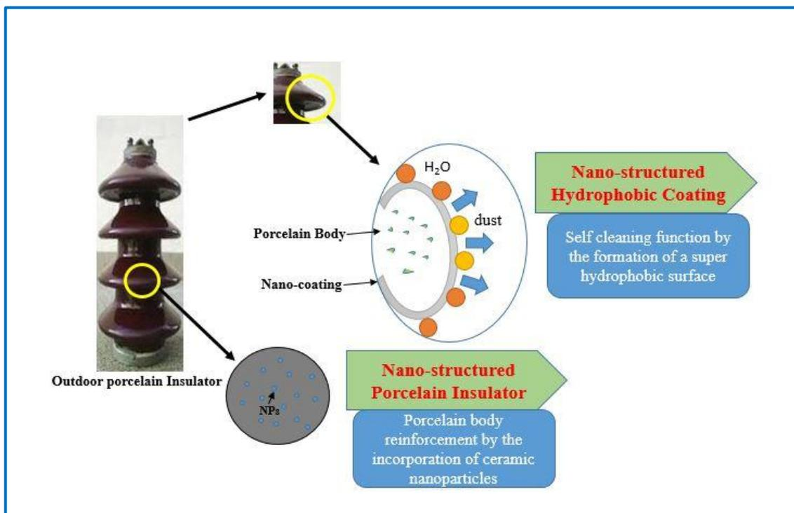
Figure 3. Schematic of the main nanotechnology concepts for outdoor insulators
