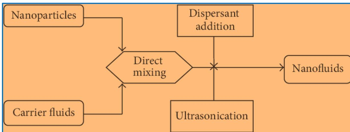
Figure 2. Preparation method of nano-fluids
