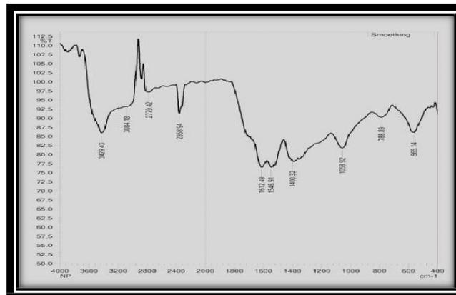
Fig. 3: FTIR Spectrum of Fe<sub>2</sub>O<sub>3</sub>
