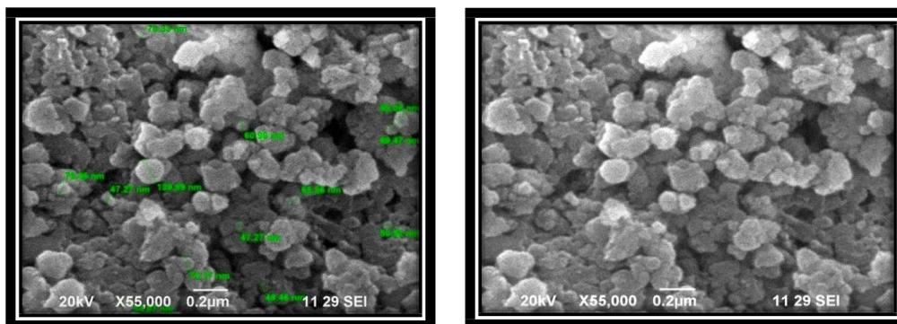
Fig. 2 SEM Images of Fe<sub>2</sub>O<sub>3</sub> Nanoparticles
