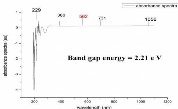
Fig. 4: UV Visible Spectra of Iron Oxide
