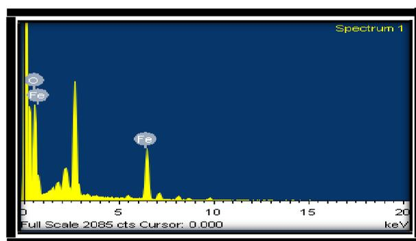
Fig. 5: EDAX of Fe<sub>2</sub>O<sub>3</sub> Nanoparticles
