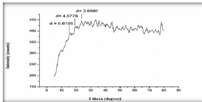
Fig.1: XRD Pattern for Fe<sub>2</sub>O<sub>3</sub> Nanoparticles
