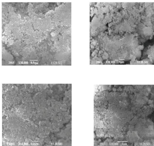
Fig. 4: SEM images of Ni doped MgO nanoparticles
