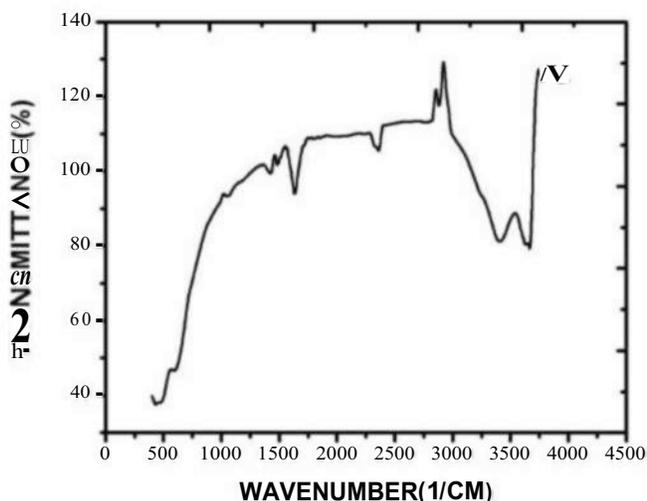
Fig. 2: FTIR image of Ni doped MgO nanoparticles
