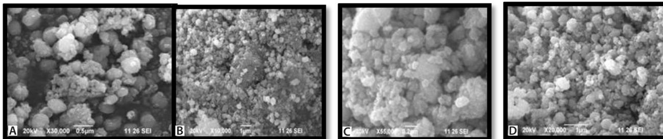
Fig. 2: SEM Images of Fe<sub>2</sub>O<sub>3</sub> nanoparticles
