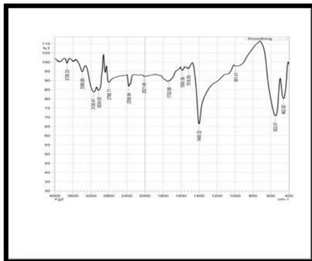
Fig. 4: FTIR vibration frequency of Iron oxide nanoparticles
