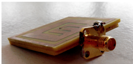
Fig.4 (a) Fabricated Structure of the antenna(Top View)
