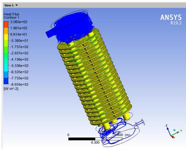
**Fig 7. Heat flux contour of cylindrical configuration**
