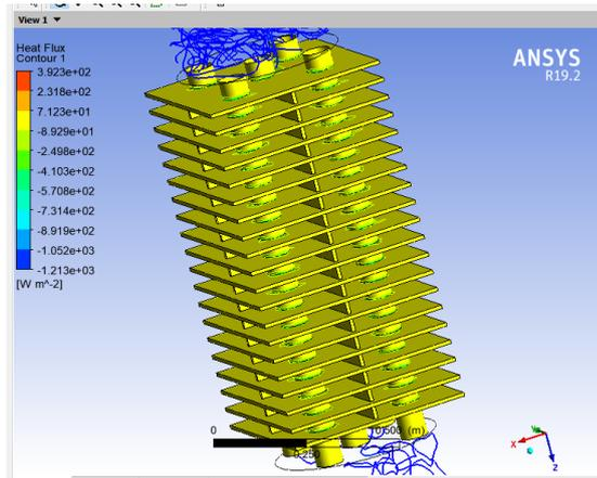
**Fig6. Heat flux contour of Square configuration**
