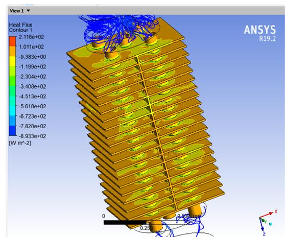
**Fig 5. Heat flux contour of Rectangular configuration**
